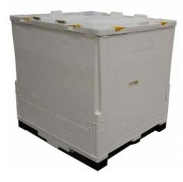
DuraGreen reusable plastic intermediate bulk containers (IBCs) make securing liquid handling safe and easy. IBCs are injection molded of FDA-approved polypropylene and have completely smooth surfaces to satisfy strict hygienic standards. These Intermediate Bulk Containers are designed to hold up to 315 gallons or 3,000 pounds of liquid and can withstand the toughest demands including filling under pressure, long-term outdoor storage, rail transport and hot fill applications.
